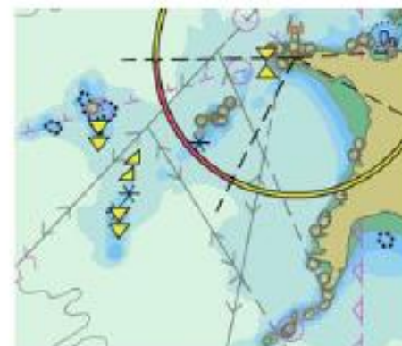
ENC displayed at 1 : 90 000 - No text displayed Note the over importance of Point LNDARE
