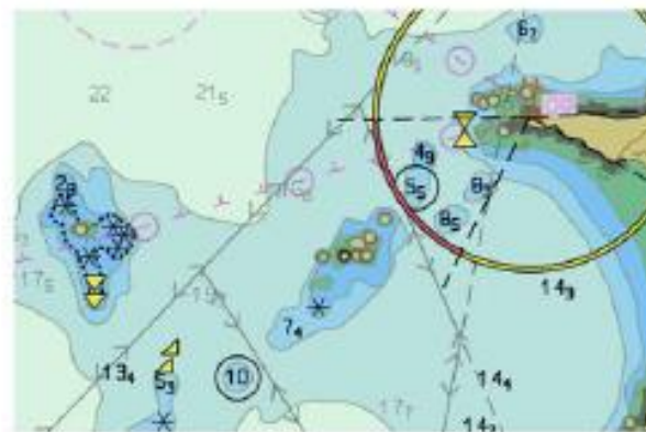
ENC displayed at 1 : 45 000 - No text displayed Overlap between objects (LNDARE, UWTROC)
